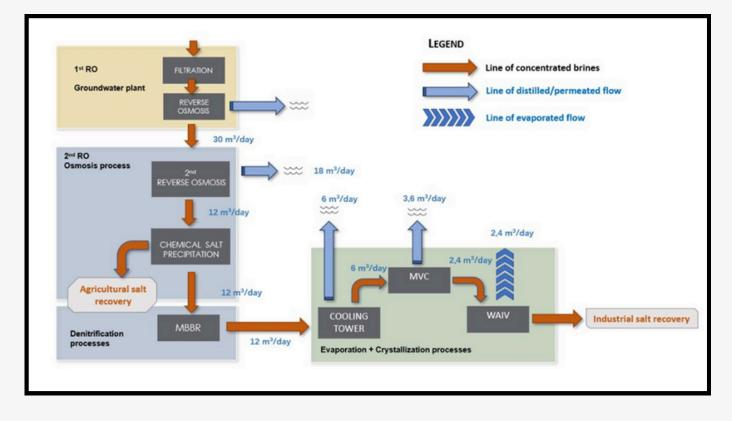
Life DESIROWS demonstration plant is designed to treat 30 m<sup>3</sup> of brine per day. The following equipment is described below:
